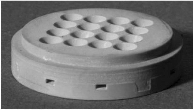
Fig. 8 Prototype 4 \times 4 mesoscale burner array fabricated in silicon nitride.
